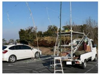
m band which my friend operated. However, because wind shook the 10 m long vertical vigorously, the antenna gave SWR of 1.1 to infinite. It was not possible to use this antenna.
