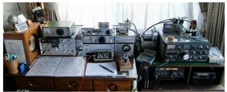
My cheap shack. From left to right: QP-7+VFO & TRIO JR-599 (1969), RX7-DX & QP-7/XTAL, 10 W power amplifier, and TRIO TS-820V (1974).
