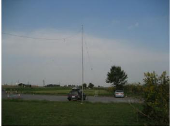
Dipole antenna 3.5MHz-28MHz
